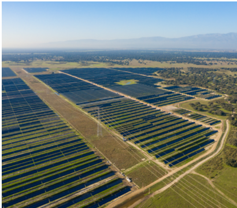
The 300 MW photovoltaic plant in Talayuela (Spain) is the largest PPA project completed by Encavis to date.
